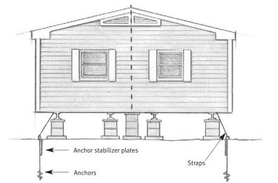
**Figure 3.5** Steel straps wrap a home's chassis beams and are held in place by ground anchors. Stabilizer plates reduce movement of the anchor head.
