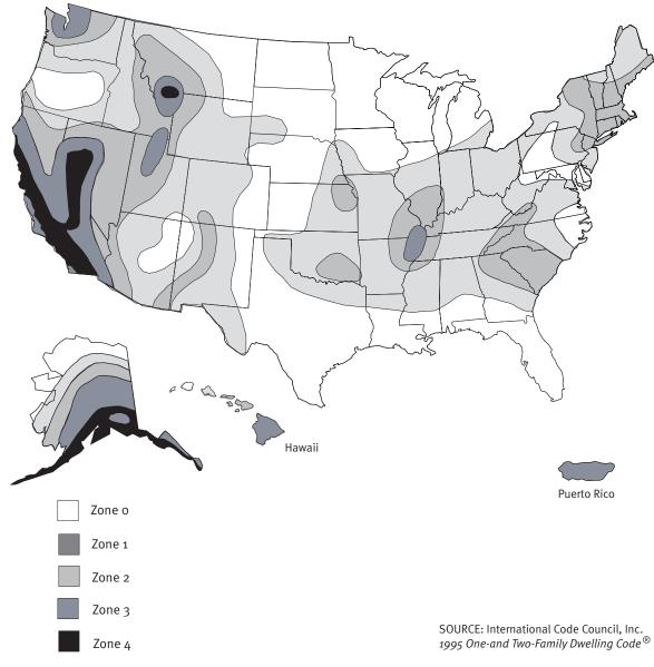
Figure 2.6 Seismic Zone Map
