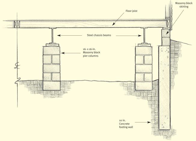
Figure 3.23 Cross section showing masonry pier supports and deep concrete perimeter wall.
