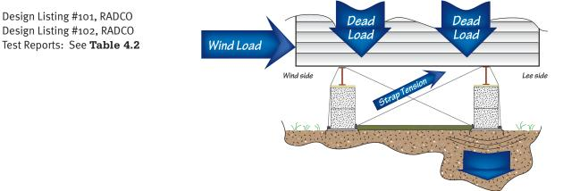
Figure 4.35 The dynamics of the Vector system.
