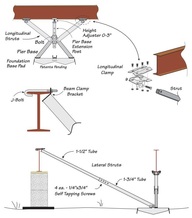
Figure 4.41 All components hot galvanized coated.
