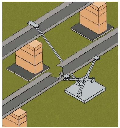
Figure 4.1 All Steel Foundation Model #1100.
