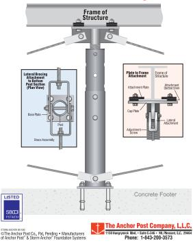
Figure 4.29 Storm Anchor details.
