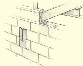
Figure 3.73 Detail of basement wall showing pocket for I-beams.
