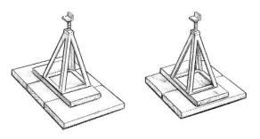
Figure 3.4. Triple and double pad footings.
