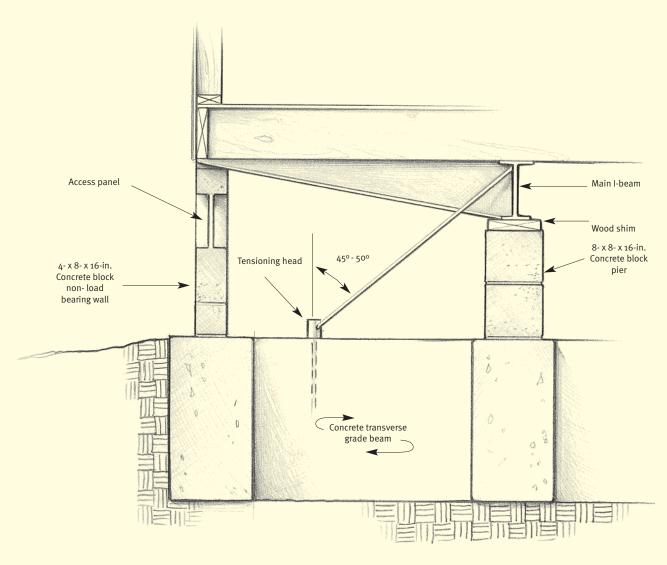
Figure 3.33 The Goff system combines a concrete slab with traditional anchors.
