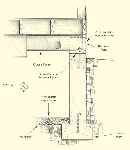
Figure 3.43 The reinforced I-beams transfer the loads to the perimeter foundation wall.
